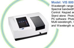
Wavelength range : 320-1100 nm Spectral bandwidth: 2 nm Control: Keypad and Software Stand alone: Photometric, Quantitative, PC software: Photometric, Quantitative, Multi-wavelength, Kinetics, DNA/Protein and Wavelength scanning
