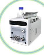
Model: Mini LC-80 Type : HPLC Flow rate range: 0.001-5.000 mL/min Maximum output pressure : 5,800 psi Detector support : UV-VIS Type of pump : Isocratic
