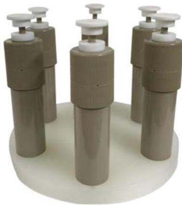
Sample digestion vessels are made of imported TFM material while outer protection vessels are made of PEEK and glass fiber which prevents high pressure and high temperature and also avoids acid, alkali as well as some organic acid.
